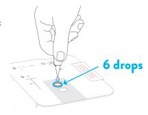
**Note**: False negative result may occur if less than 6 drops of fluid are put in the hole.
